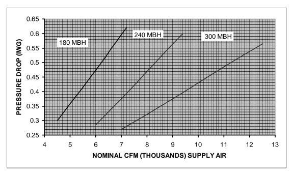
FIGURE 18 - PRESSURE DROP ACROSS A DRY INDOOR COIL VS SUPPLY AIR CFM FOR ALL UNIT TONNAGES
